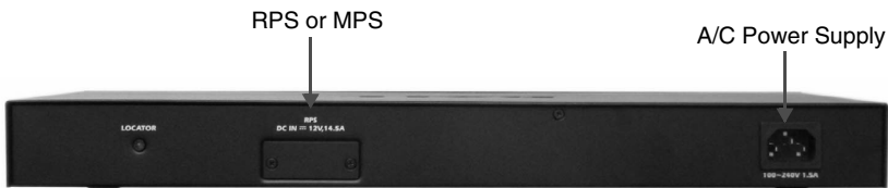
Figure 1-2. Back-Panel Power Connector
